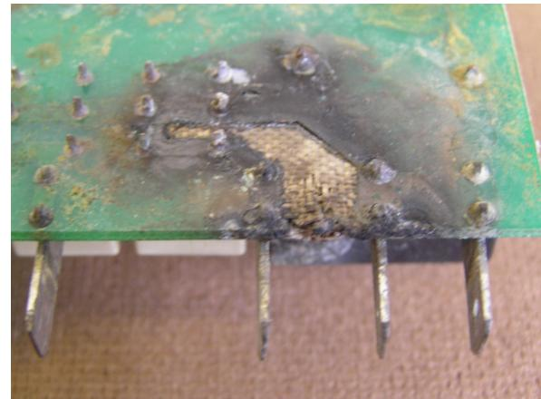
The conformal coating materials are assessed using two standards. The first is IEC 112 that is used to determine the comparative tracking index (CTI) of solid insulating materials such as conformal coatings under moisture conditions. The second is IEC 587 to measure the resistance to tracking and corrosion under more aggressive circumstances.
