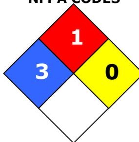
**Health and Safety:** The 834FRB parts can ignite if the liquid is heated, but once it is cured it is a self-extinguishing epoxy solid. Do not breathe in fumes of a cured epoxy block that is exposed to an external flames source because the flame retardant releases bromine to extinguish the flame.
