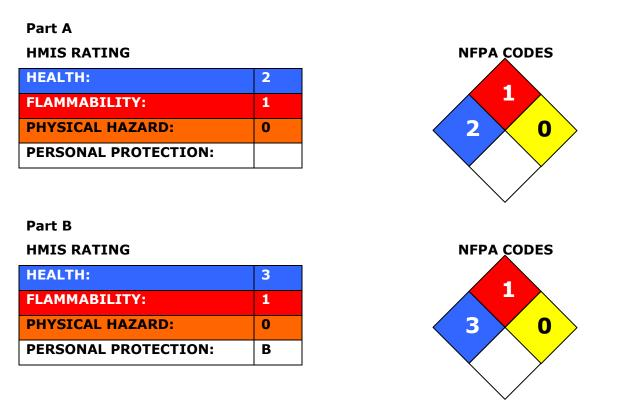
*Health and Safety:* The 832HT parts can ignite if the liquid is both heated and exposed to flames or sparks.
