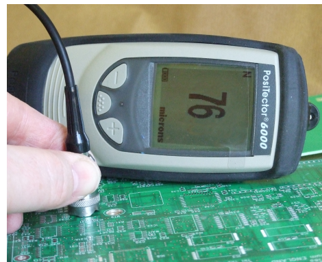
Dry Film Measurement of a conformal coating on a printed circuit board using a Positector 6000
