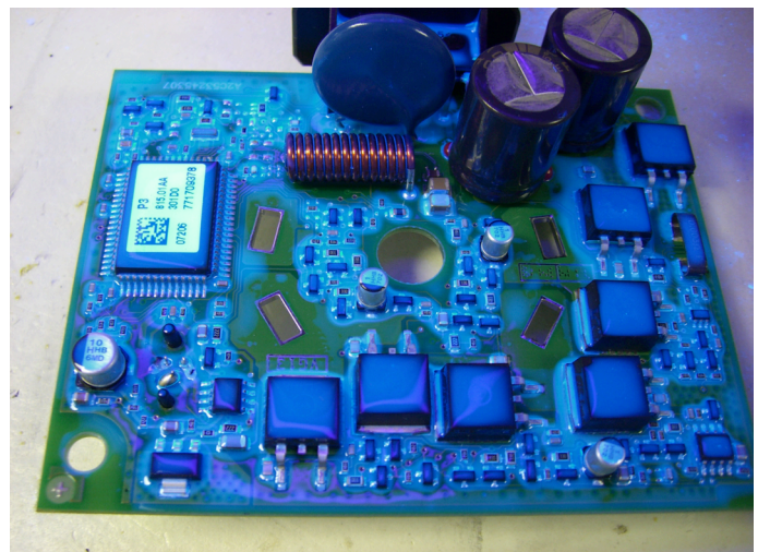
Examples of Conformal Coating Capillary Effects
