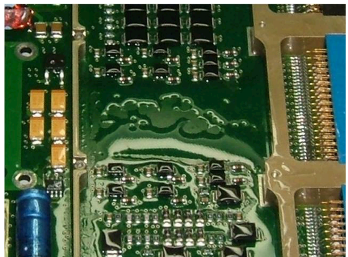
Examples of Conformal Coating De-wetting
