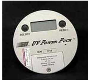
Power Puck radiometer
