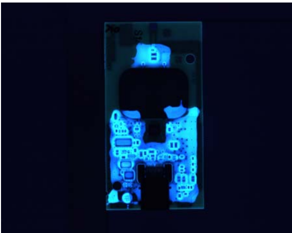
A conformal coated automated selective spray PCB
